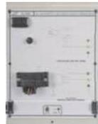
KL-84003 AIR-flow Sensor Hot Wire & Manifold Absolute Pressure Sensor
