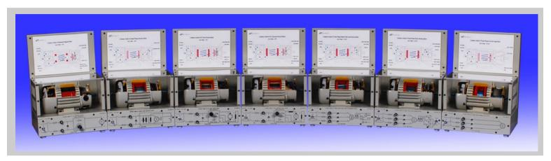
Cutaway models are made from normal electrical machines. The stator is cut away by 1/4 over the entire length to enable an optimum view of the internal construction of the machine and it is still operating. The cutaway surfaces are protected against corrosion.
