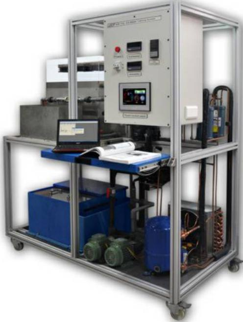
The Mini Ice Plant Training System (KR-112) provides a learning platform for students to understand various freezing methods in terms of Industrial 4.0 practice through wireless transmission and remote control, the structures of the components, and the operating principles of ice plant systems.
